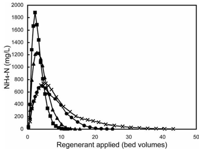
**Figure 4.** Influence of regenerant content on regeneration rate: ■ – 30 g/L NaCl; ▲ – 20 g/L NaCl; ● – 10 g/L NaCl; x – 6.24 g/L HCl.
