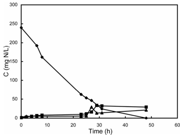
**Figure 7.** Biological nitrogen removal from regenerate of ion exchange batch test with CANON process:  $\blacklozenge$  - NH<sub>4</sub>-N  $\blacksquare$  - NO<sub>2</sub>-N;  $\blacktriangle$  - NO<sub>3</sub>-N.
