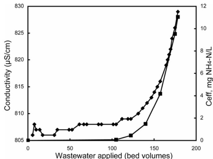
**Figure. 5.** Ion exchange column exhaustion with real wastewater: ■ – C<sub>eff</sub>, ♦ - Conductivity.
