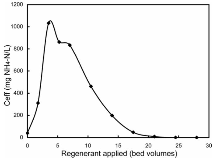
**Figure 6.** Ion exchange column regeneration with 10 g/L NaCl solution.
