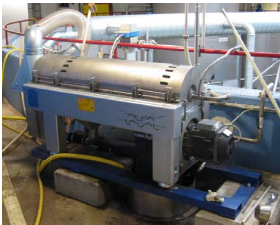
Figure 4. Decanter centrifuge for sludge dewatering.
