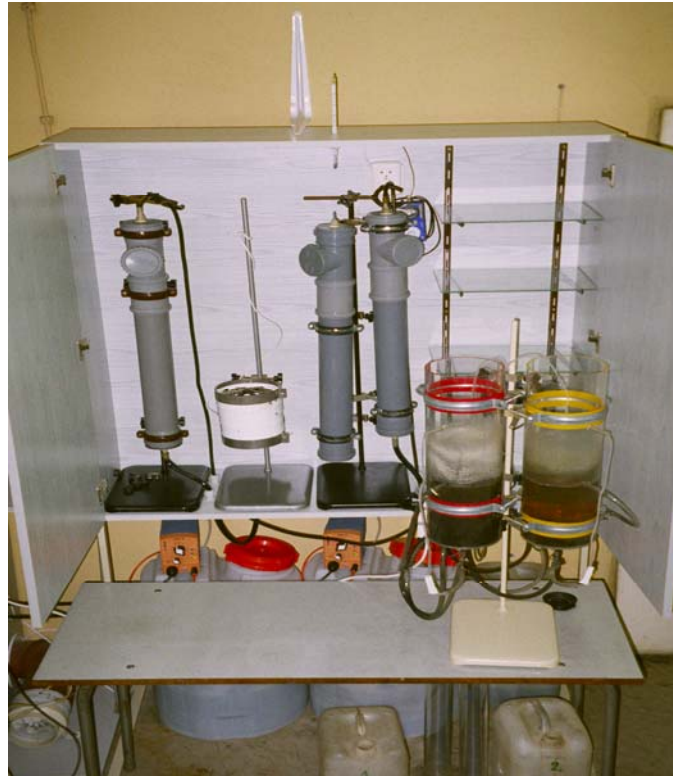
Figure 2. Laboratory system of the anaerobic-aerobic textile wastewater treatment.
