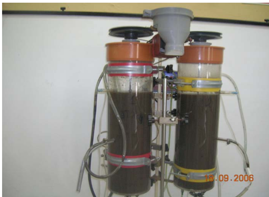
Figure 1. Laboratory biological sewage treatment reactors.
