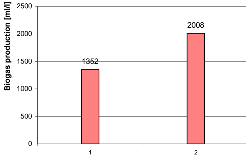
Fig. 6. Effects of anaerobic digestion for 17 days of (1) activated sludge (blank) and (2) with addition of 20 % disintegrated sludge.
