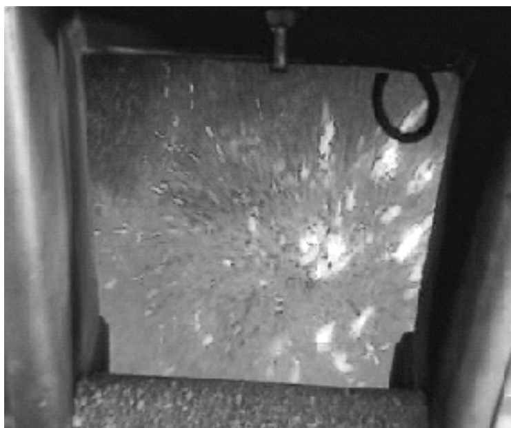
Figure 3. The combustion of solid fuel in the semi - technical scale fluidised bed reactor, 100 kW.
