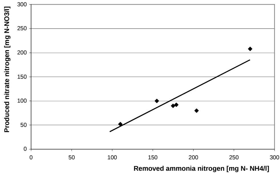
Figure 2. Correlation between removed ammonia and nitrates produced.
