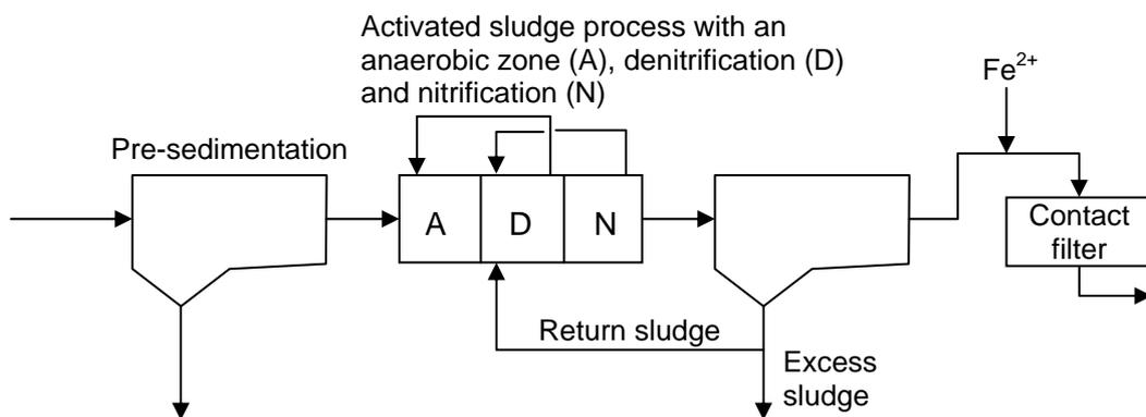
**Figure 2.** Process schedule for a main stream process with pre-sedimentation, biological phosphorus and nitrogen removal (UCT-process) and contact filter.
