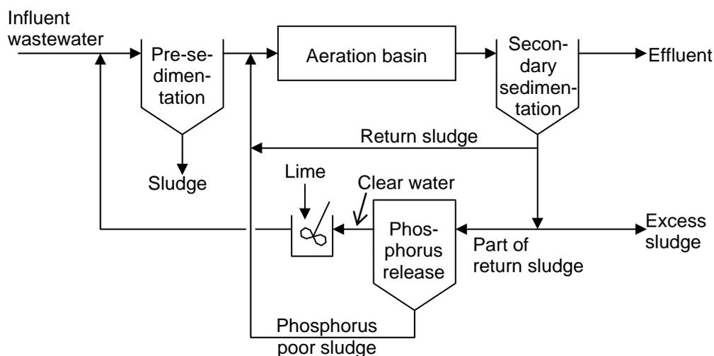
**Figure 3.** Schematic process scheme of PhoStrip (Drnevich, 1979).
