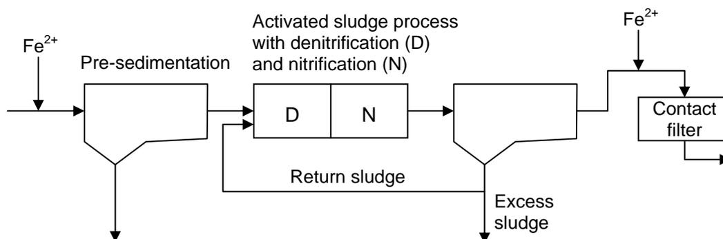
**Figure 1.** Process schedule with pre-sedimentation, pre-denitrification and contact filter.
