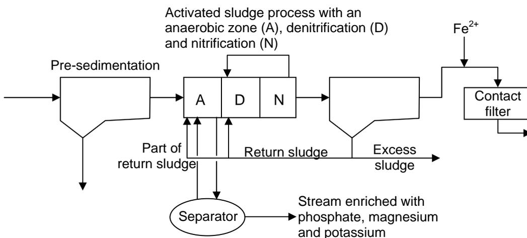
**Figure 4.** Process scheme with a side-stream process for biological phosphorus recovery with pre-sedimentation, biological phosphorus and nitrogen removal and contact filter.
