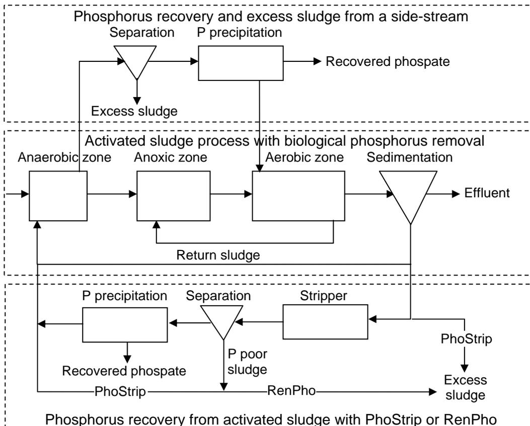
**Figure 7.** Different system technology for recovery of phosphate from phosphorus rich side-streams.
