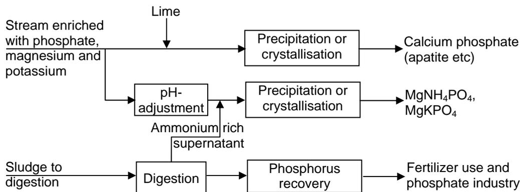
**Figure 6.** Two-stage phosphorus recovery process based on process technologies in figure 4 and 5.
