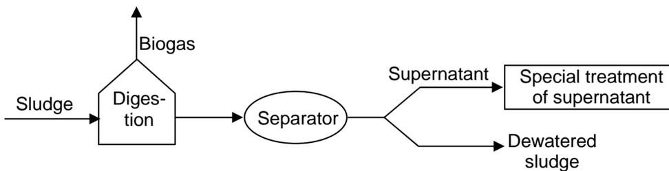
**Figure 5.** System for treatment of sludge with digestion followed by possibilities of separate treatment of supernatant.
